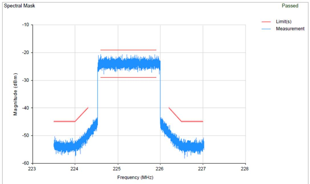
Figure 21: Waveform Limit Test Result (PDF Report)
