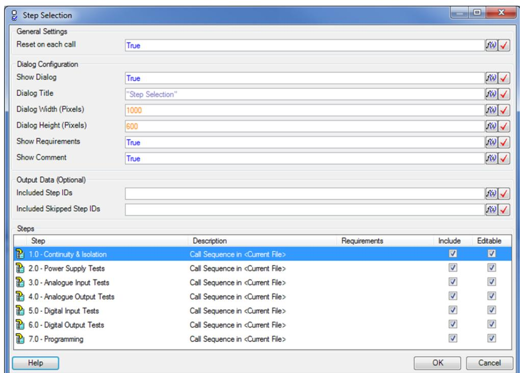
At run-time, a simple window will be displayed to the operator giving the option to skip particular steps before executing or terminate the sequence. An example is shown in Figure 24. Steps displayed in the dialog will match those which have the “Include” flag set in the configuration. Those with “Editable” set to false cannot be modified by the operator.
