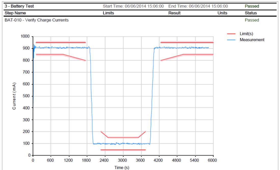
Figure 20: Waveform Limit Test Result (PDF Report)
